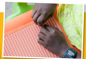
A plastic template with squares that the paper is inserted into to write with the stylus.
