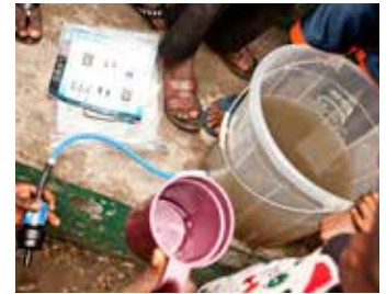
The filter makes the dirty water drinkable.
