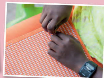
A plastic template with squares that the paper is inserted into to write with the stylus.
